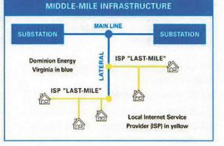
Main Line is the communication line between substantons Lateral is the communication line that connects to a main line
